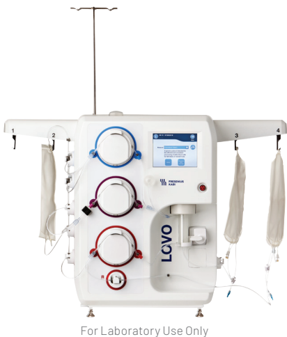
Figure 1: Depiction of the spinning-membrane cell washing instrument.
